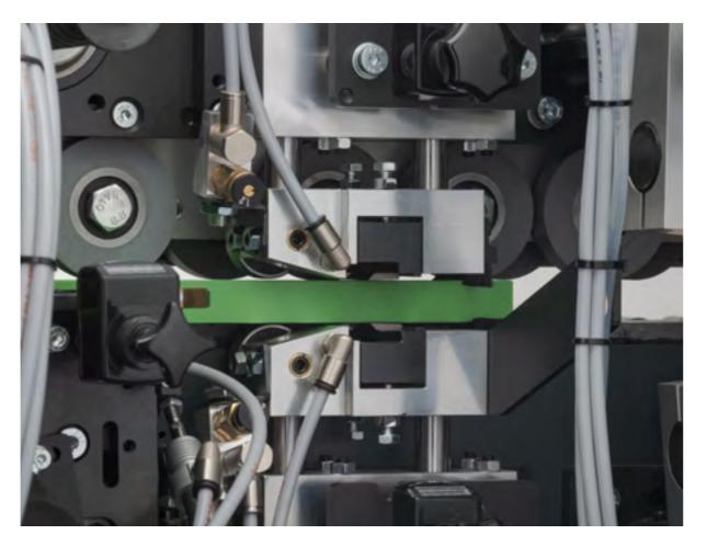
**Surface scraper:** Dynamically stored flat scraper ensures high production quality even for difficult materials. The wide contact surface precisely and gently scans the edge material to ensure consistent quality and removes adhesive residue and excess edges.
