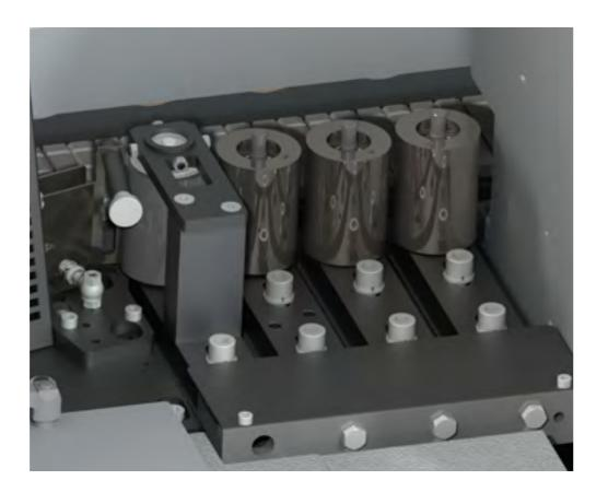
**8 mm execution:** The maximum edge thickness increases from 3 mm to 8 mm. Process real wood edges with more powerful motors and increase the lifespan of your tools. **KXX/01**
