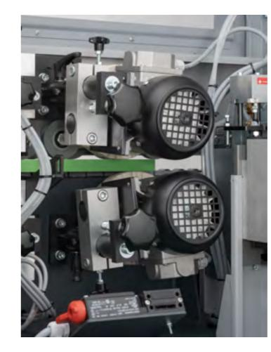
Cleaning station: The two polishing discs free the upper and lower panel from excess sprays, adhesive residue and lighten in the event of edge stress whitening. 2 x 0.18 kW motors, individually adjustable for consistent cleaning results when using various processing technologies.
