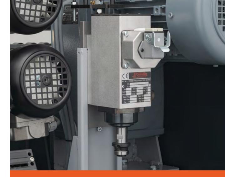
Changeable motor for corner rounding: The preset interchangeable motor including tool allocation reduces machine set-up time when changing the front head radius. The quick-change preliminary setup allows the motor to be changed quickly without the need for any additional settings.
