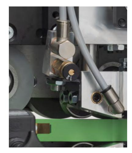
Cleaning agent spraying unit: This spray system applies the cleaning agent to the top and bottom of the workpiece. Applying the cleaning agent followed by the cleaning station removes any sprays, adhesives and impurities.
