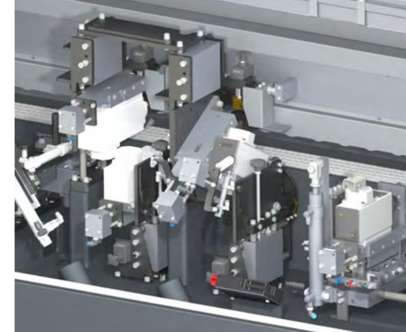
**2nd milling station:** Thanks to the second milling station, you can produce various radiuses with greater flexibility. Greater chip weights can be realised thanks to pre-milling and precision milling. A 30° chamfer can also be produced by manually adjusting the unit.
