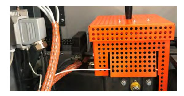
**Glue level sensor:** The optional glue level sensor for your interchangeable glue pots lets you keep track of things and avoid stoppages and gluing errors. The user is notified of low levels in good time via plain text notifications. **KXX/36**
