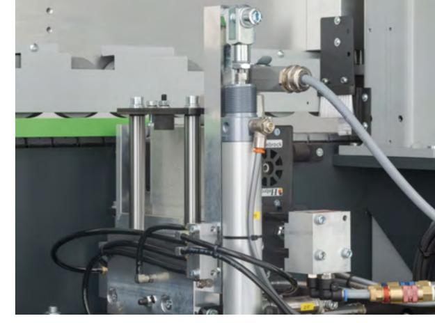
**Corner rounding unit:** The corner rounding optimally prepares you for any challenge when it comes to dealing with the front of the turning heads. Thanks to intelligent programming via the touchscreen display, individual sides and processing settings can be set. Whether it's the front and/or rear edge, radius or chamfer settings or choosing between an entire side or only the vertical edge, there are no limits here.
