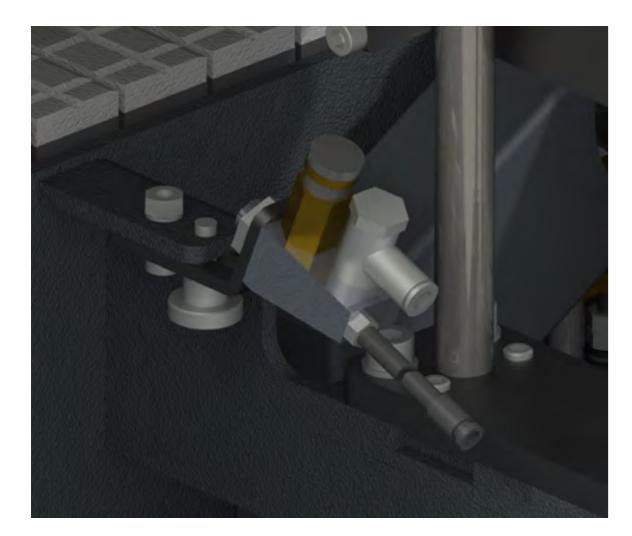
**Protection spraying edge:** The additional nozzle sprays the lubricant laterally over the edge banding surface. The wetted edge/film then further transports the lubricant.
