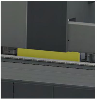
Heatable infeed fence: This option allows panel materials to be heated prior to processing to reach the optimum processing temperature. Recommended for temperature fluctuations in workshops or outdoor warehouses where the materials are stored.
