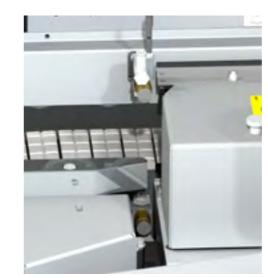
**Release agent spraying unit:** Prior to edging, the spray system casts a fine layer of separating agent over the top and bottom of the workpiece edges.
