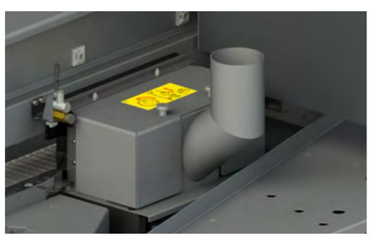
**Pre-milling (Whispercut):** The WhisperCut pre-milling system with interchangeable diamond cutter tips ensures maximum tool life (manual height adjustment) and tear-free milling results due to an oblique cut through the centre of the panel. Two ready-to-use cutter heads guarantee tear-free milling results, even for demanding materials and surfaces.
