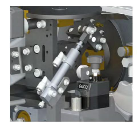
**Multi-radius scraper:** The multi-radius scraper allows you to process R2 and R1 radii without having to change the machine settings for flexible processing of different radii. The radius settings can be individually selected or saved as a programme.
