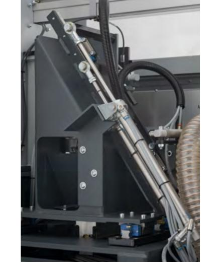
**Double motor trim saw system:** The stable design of the double motor trim saw unit with linear guides enables precise milling of the front and/or rear workpiece, including for high unit quantities and small workpiece sequences. The cross-cut saws can be adjusted by 12.5° as required. Simply choose the setting via the touchscreen display on the front of the machine.
