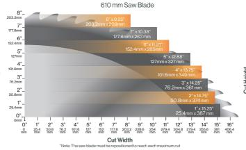
TigerSaw MiterXL - Cutting Envelope at 45° 610 mm Saw Blade
