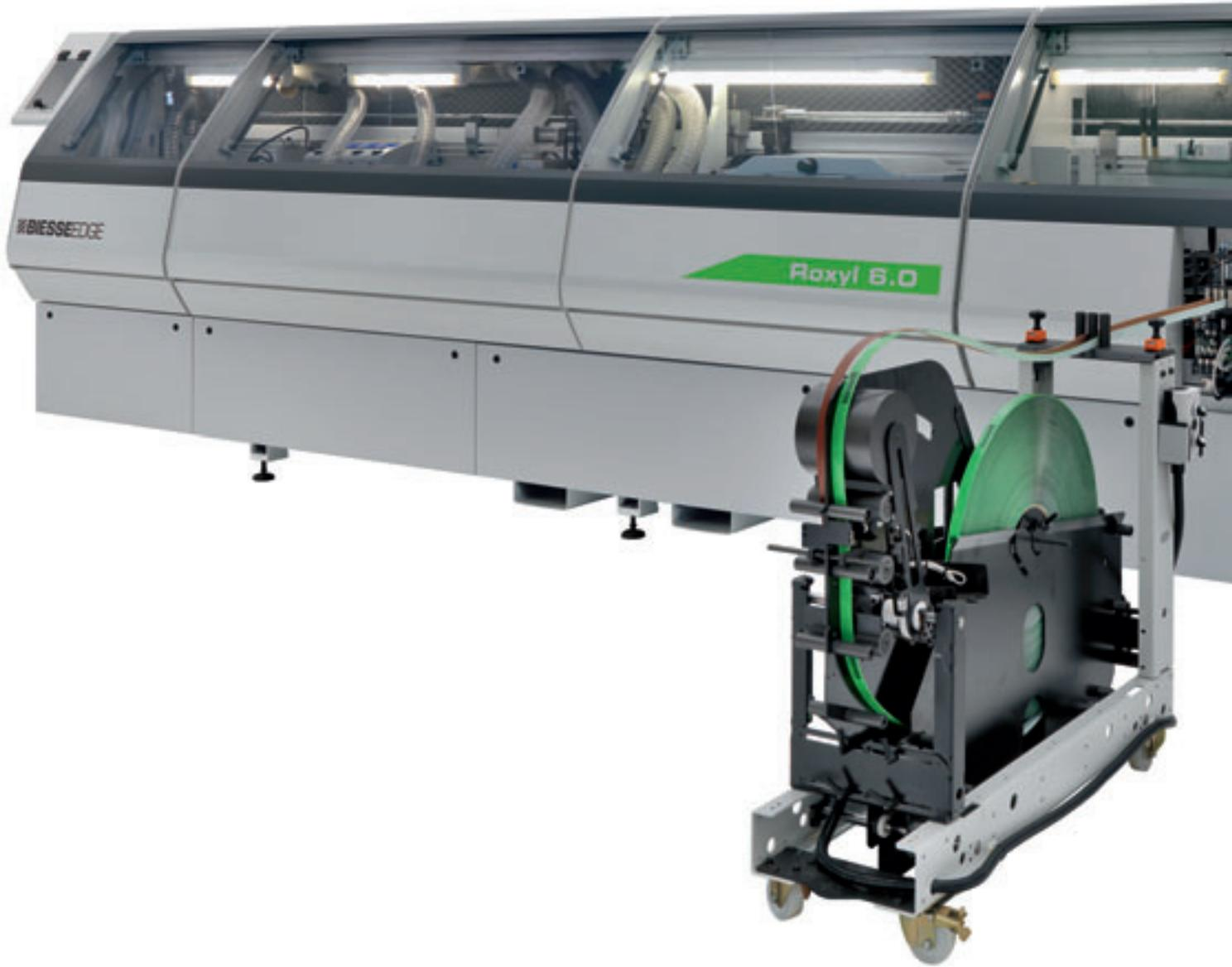
Roxyl is a range of automatic, industrial edgebanding machines designed to create a new standard in automatic edgebanding. An innovative, modern, ergonomic design is combined with productivity, efficiency and flexibility for the application of all types of edge-banding material. The control system uses either a high level NC system or a Personal Computer.
