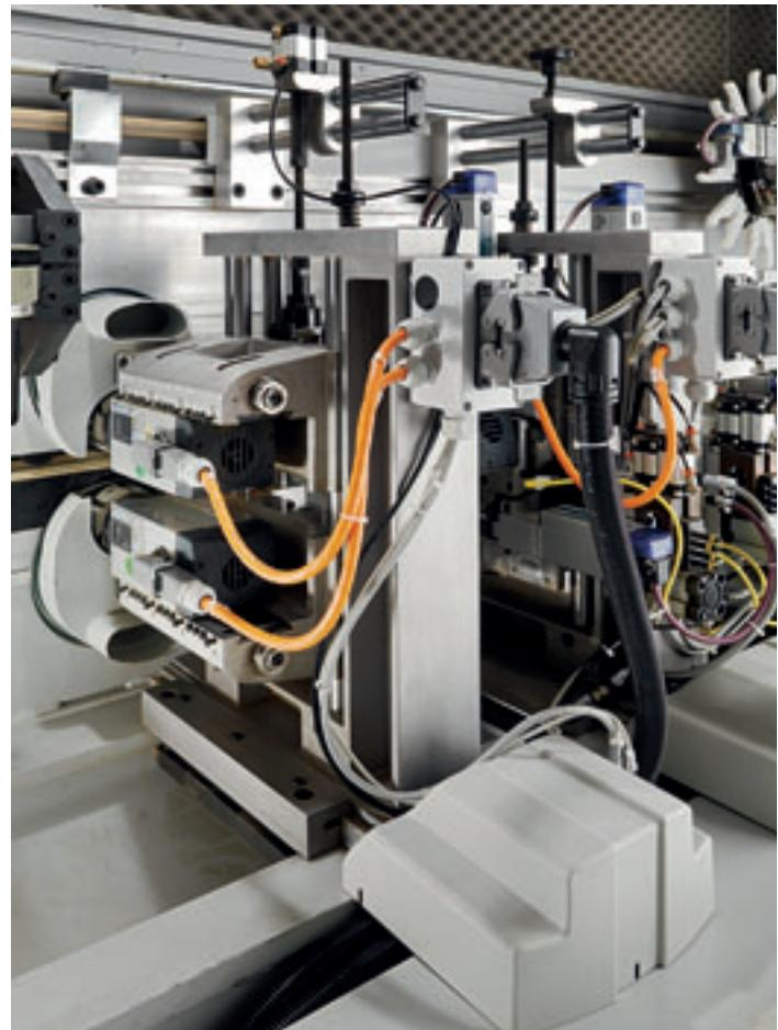
Top and bottom edge trimming unit RS-100.
