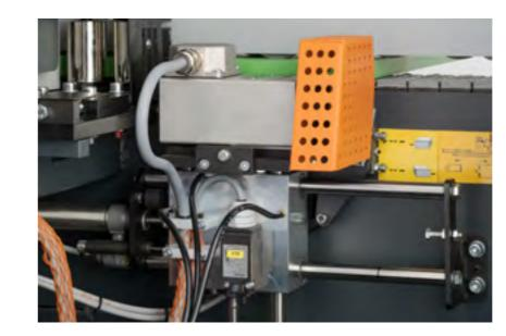
**Trim saw station:** The stable design of the single-motor cross-cut saw with linear guides enables precise sawing of the front and rear workpieces. Simply choose the setting via the touchscreen display on the front of the machine.
