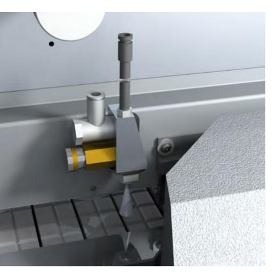
**Release agent spraying unit:** By applying the separating agent to the top and bottom of the workpiece, this prevents any excess adhesive residue from sticking to the workpiece Prior to edging, the spray system casts a fine layer of separating agent over the top and bottom of the workpiece edges. This prevents any excess adhesive from sticking to the workpiece. This option is recommended if regularly working with PUR adhesives.
