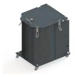
**PUR box:** Our PUR box slows down the hardening of PUR adhesive in glue pots by using a compressed air drying process, increasing the potential processing time of the adhesive up to 7 days before cleaning is required. This accessory is recommended if regularly working with PUR adhesives.
