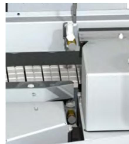
**Release agent spraying unit:** Prior to edging, the spray system casts a fine layer of separating agent over the top and bottom of the workpiece edges.
