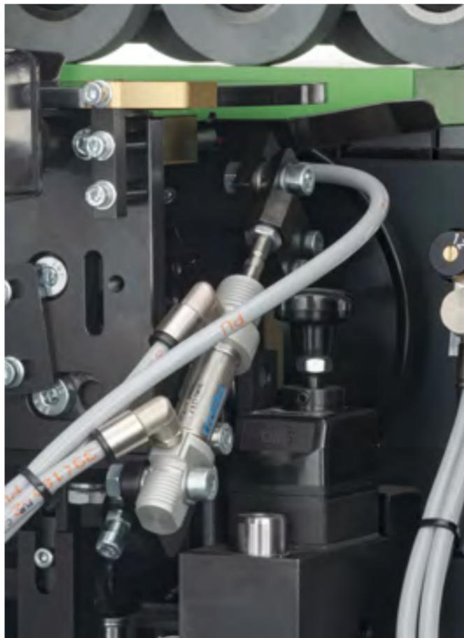
**Nesting for milling station and radius profile scraper:** Allows working with tool sharpening and hinge hole drilling with a milling unit and radius scraper. The settings can be easily changed via the display on the front of the machine. Scanning of the workpieces takes place underneath the panel.
