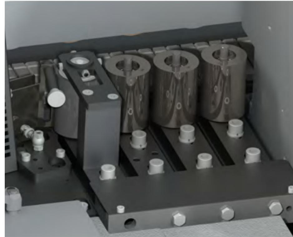
**Heatable infeed fence:** This option allows panel materials to be heated prior to processing to reach the optimum processing temperature. Recommended for temperature fluctuations in workshops or outdoor warehouses where the materials are stored.
