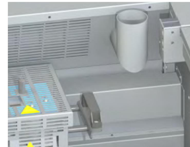
**Glue pot suction hood:** A special hood above the glue pot allows toxic steam to be diverted away via an external extraction system and improve the air quality inside your workshop.
