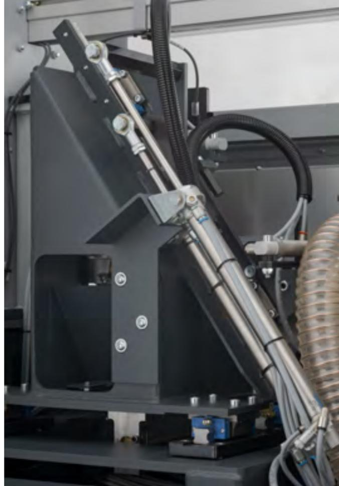
**Double motor trim saw system:** The stable design of the double motor trim saw unit with linear guides enables precise milling of the front and/or rear workpiece, including for high unit quantities and small workpiece sequences. The cross-cut saws can be adjusted by 12.5° as required. Simply choose the setting via the touchscreen display on the front of the machine.
