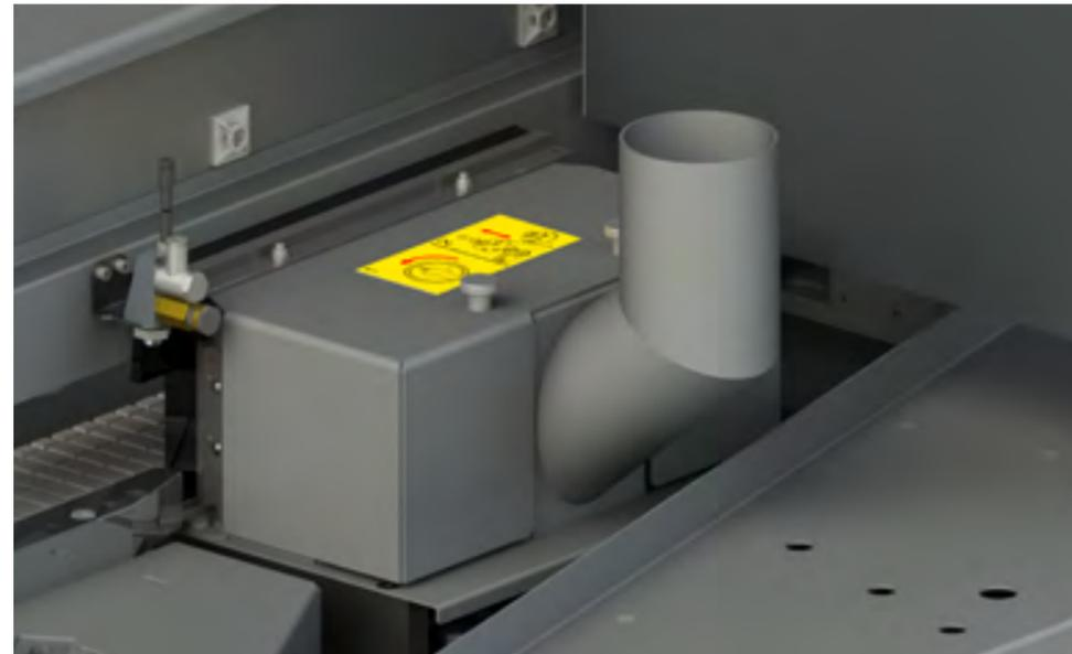
**Pre-milling (Whispercut):** The WhisperCut pre-milling system with interchangeable diamond cutter tips ensures maximum tool life (manual height adjustment) and tear-free milling results due to an oblique cut through the centre of the panel. Two ready-to-use cutter heads guarantee tear-free milling results, even for demanding materials and surfaces.
