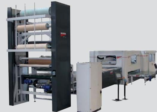
**2-roll PVC foil dispenser with automatic cut-off device**
